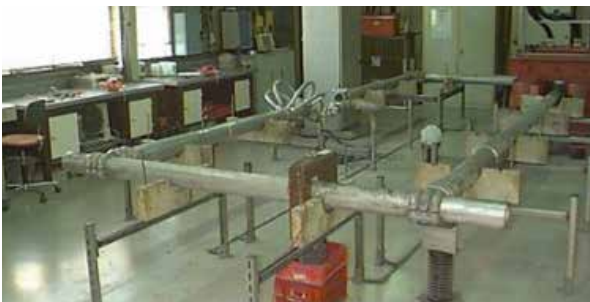
Temperature rise test up to 10 kA
