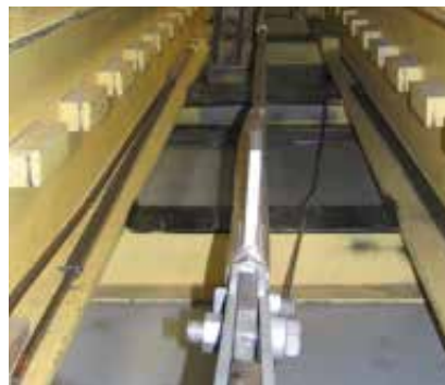
Tensile test up to 70 T
