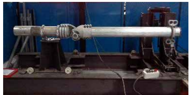
Cantilever/Bending test up to 5 T/Axis
